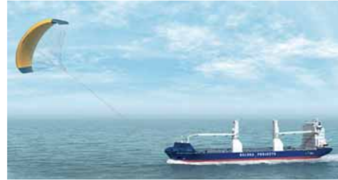
Environmentally friendly wind propulsion system for future ships: The SkySails system uses a large towing kite similar to a paraglider to propel cargo vessels, superyachts and fish trawlers.
