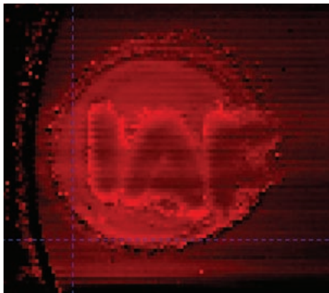
Image of an inhomogeneous surface coating with TNT taken using the IRLDEX process (source: IRLDEX)
