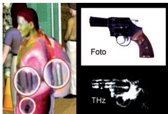
Checkpoint scenario and experimental THz image made within ten seconds of a weapon hidden under clothing (source: GE (left); Uni-FFm / RPG)
