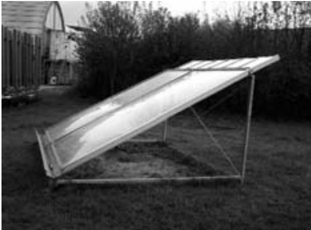
Fig. 1: Test stand at Research Center Jülich for weathering test of different cover materials, in particular glass foil combination
