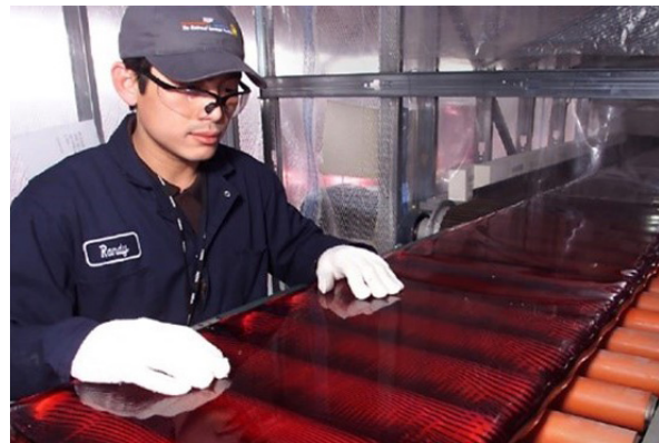
Fig. 20: NIF laser facility (left), continuous strip of laser glass exiting the melter at NIF (right).
