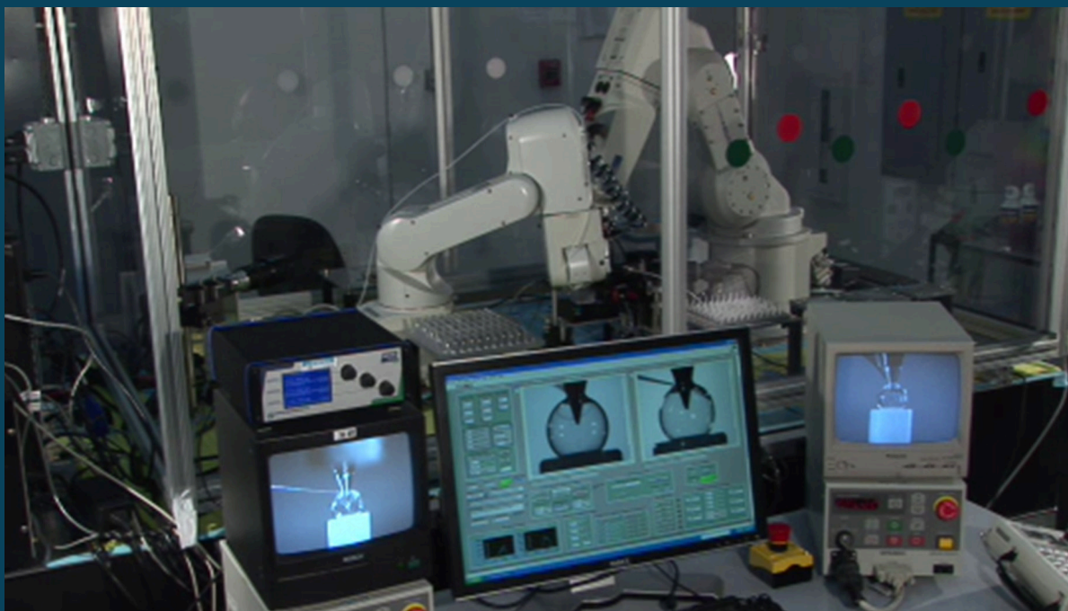
Fig. 11: Robots set up and programmed to assemble cone-in-shell targets at General Atomics. Cone tips centered to capsule center to within +/- 10 microns. Courtesy of General Atomics.
