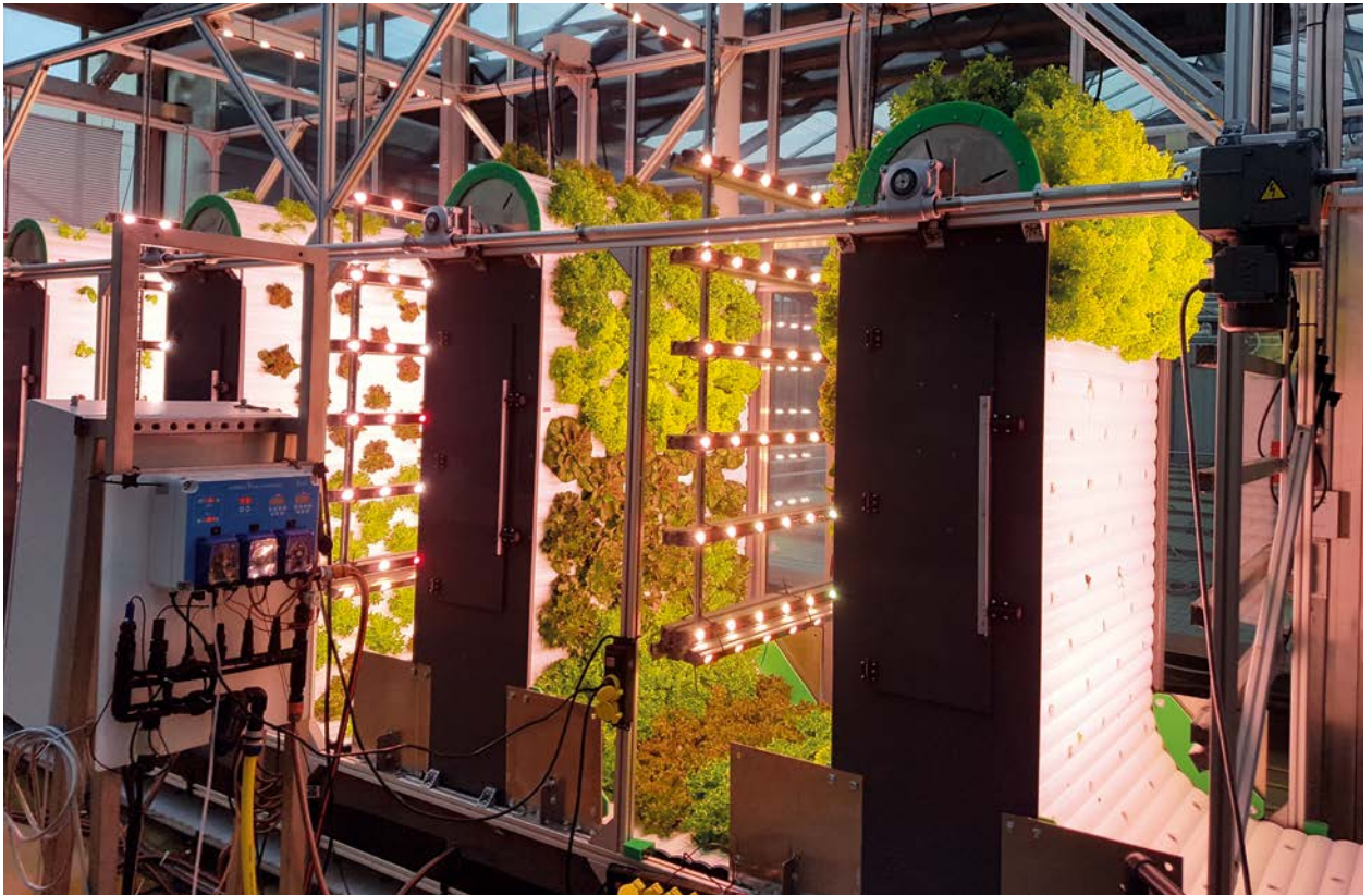
Salad from the assembly line: The automated, vertical plant cultivation system OrbiPlant at the Fraunhofer IME in Aachen.
