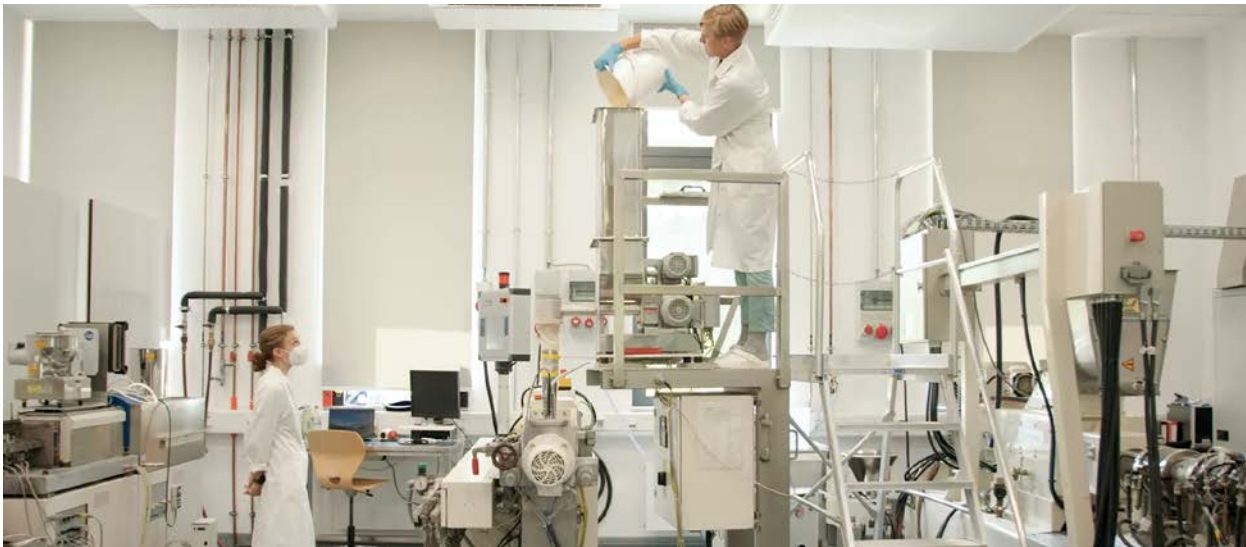
Lupine seeds are processed in the extruder plant at the Fraunhofer Institute for Process Engineering and Packaging in Freising.
