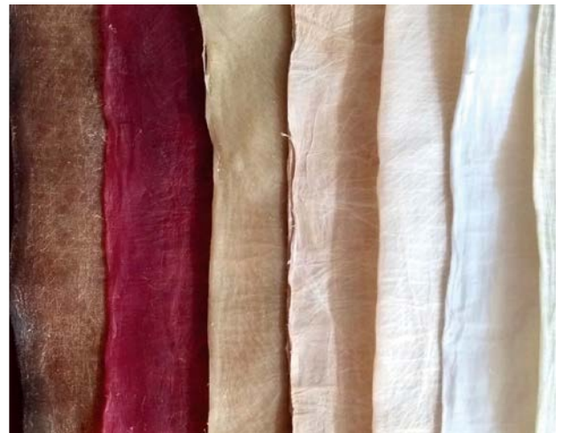
AMSilk produces textile fibres from microbially produced spider silk proteins (left). Imitation leather made from bacterial nanocellulose by ScobyTec (right).
