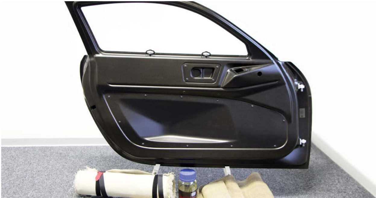
Biogenic fibres, resins and varnishes are used at the Fraunhofer Institute for Wood Research (WKI) to create lightweight components for the Bioconcept Car.
