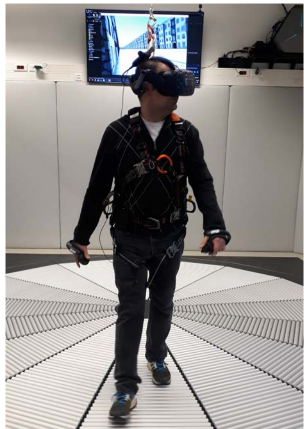
Pedestrian Simulator at German Aerospace Center (DLR): Simulating urban traffic scenarios in virtual reality.
