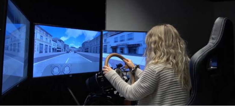
Driving Simulator at Ulm University: A person is driving manually while encountering a bottle-neck scenario in an urban area.
